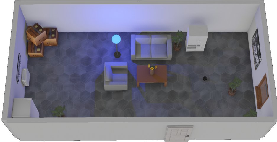
Figure 7.12: Webots world used to verify TurtleBot3 Burger mapping and navigation capabilities
